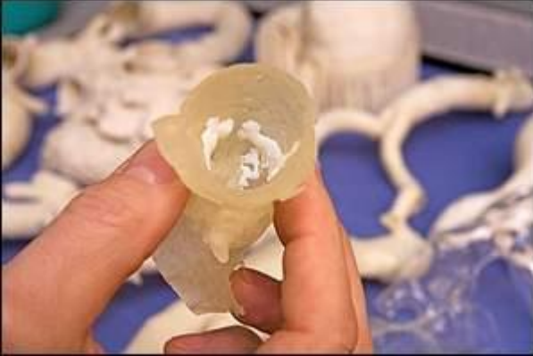
Mr. West holds an aortic valve with calcification created by the shop's Connex 3D printer.
